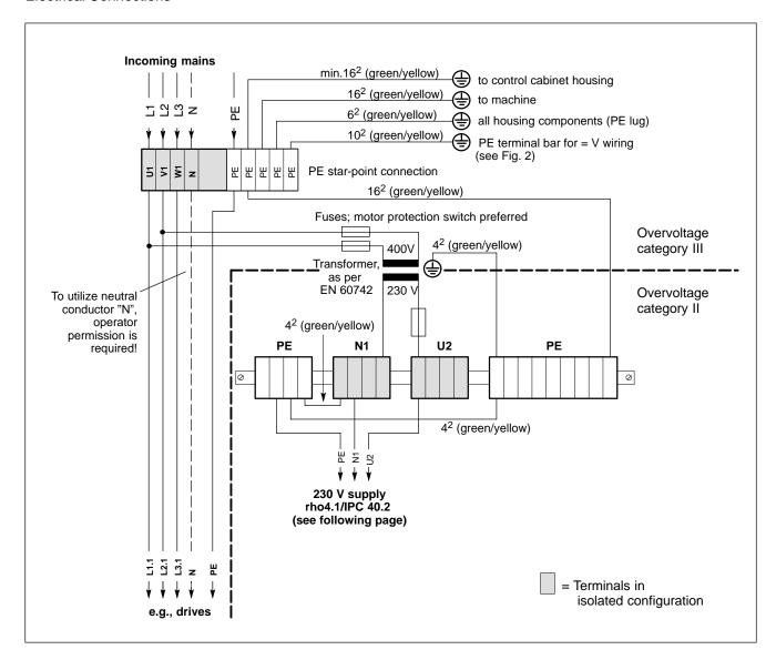
Power connection 230 VAC via separation transformer
