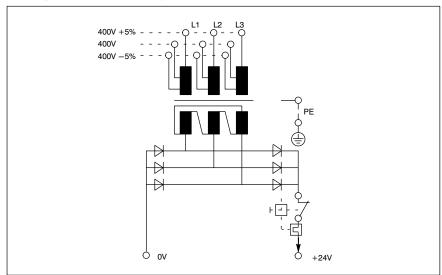
Offset AC components of the type produced by an unregulated rotary current bridge circuit without smoothing, with a ripple factor of 5% (refer to DIN 40110/10.75, section 1.2), are permissible. As an upper voltage limit, this produces a maximum absolute value of 30.2 V and, as a minimum voltage limit, the minimum absolute value of 18.5 V.
