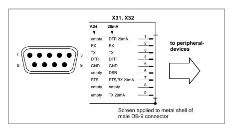
The X35 PHG connector and the X31 serial interface port must never be in use, i.e., connected, at the same time.
