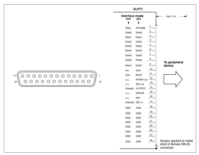
The parallel port normally runs in the default SPP (Standard Parallel Port) mode. Provided that suitable peripheral devices are present, it can also be operated in EPP (Enhanced Parallel Port) or ECP (Extended Capabilities Port) mode. The mode is changed by means of the BIOS settings.
