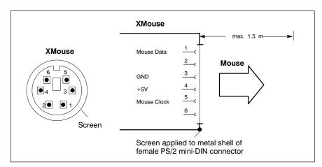
If the P/S2 mouse is not recognized by the system, it must be enabled in the BIOS by switching from Disabled to "Autodetect".
