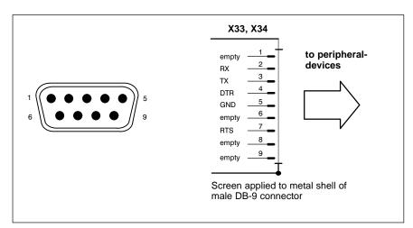
Connecting cable between X31..X34 connectors and an external PC (e.g., for ROPS4 coupling).
